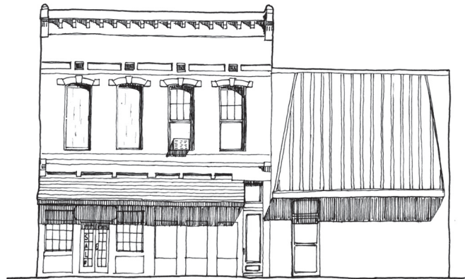
On the left: boarded-up windows, a chopped-up storefront with inappropriate multi-paned colonial-style windows, and a poorly designed awning. On the right: a windowless first floor, and an oversized “awning.”
