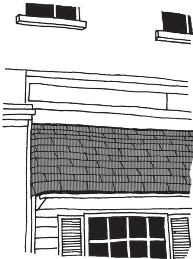
Storefront opening filled with a colonial-style insert. The asphalt shingles, multi-paned windows, clapboard siding, shutters and other residential features and materials are not appropriate for downtown commercial buildings.
