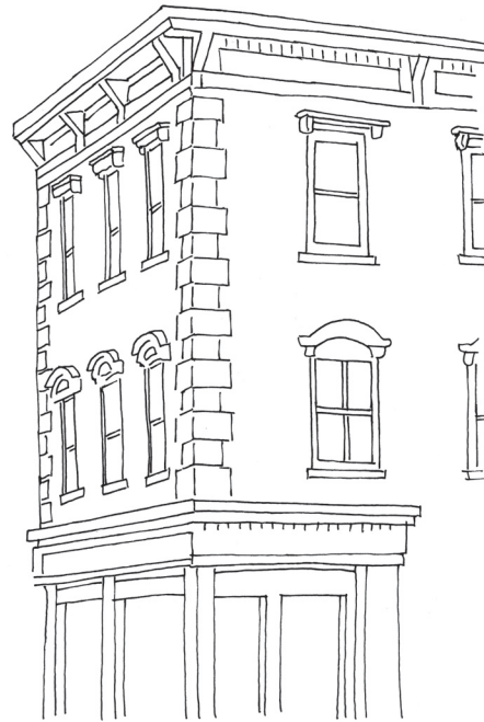
The upper facade typically has expanses of flat wall punctuated by windows. The storefront, in contrast, is mostly display windows and doors with thin framing around them.
